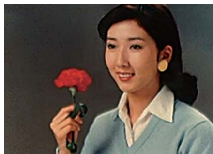
Fig. 10 Photograph of a skin color chart, which was taken by the trial product of the proposed organic CMOS sensor with micro color filters.
