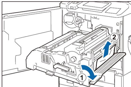
8. Open the handle [2f] right and remove the jammed paper.
