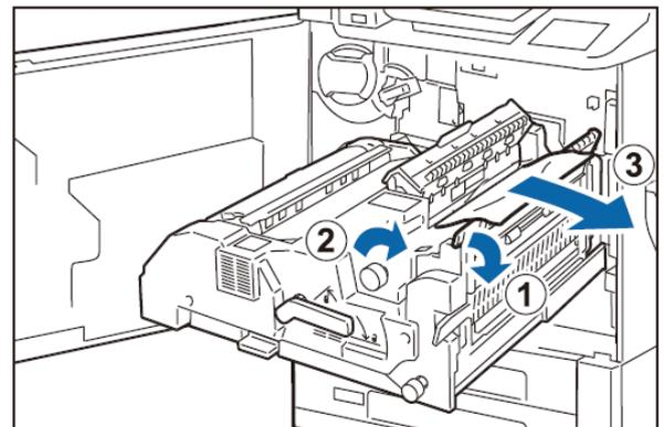
7. Open the handle [2e] and remove the jammed paper.
