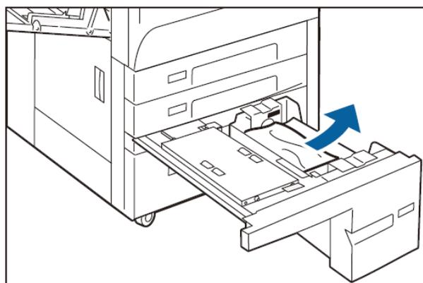
3. If paper is jammed in the paper feed section, open the inner cover and remove the jammed paper.
