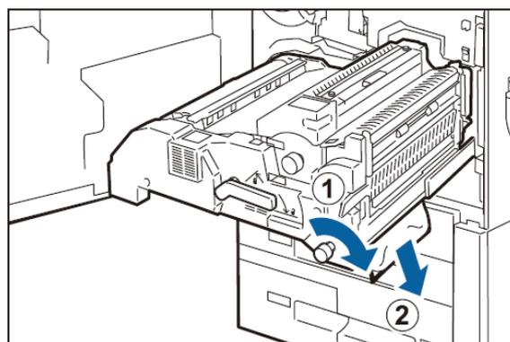
9. Open the handle [2g] and remove the jammed paper.
