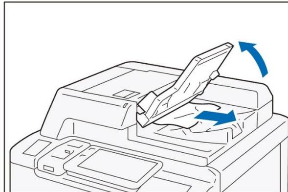
5. Open the Document Cover, pull down the handle to open the Side 2 scanner, and then remove the document.
