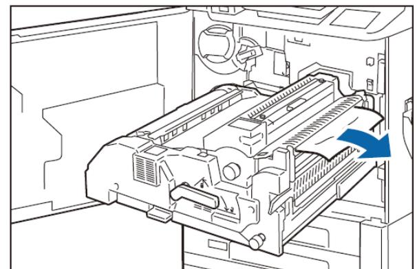
4. Open the handle [2a] (1) and remove the jammed paper (2).
