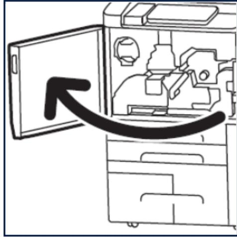
2. Open the waste toner cover at the bottom right side of the device.
