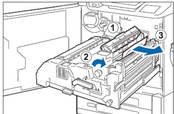
6. Open the handle [2d] right (1), turn the knob [2c] right (2) and remove the jammed paper (3).
