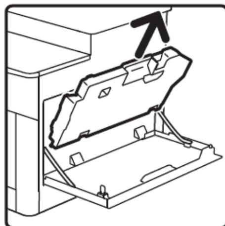
4. Make sure that the two indented parts on the bottom go into the brackets on the printer.
