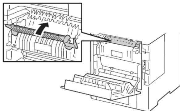
5. Open the paper guide on the fusing unit.
