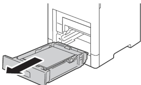
4. Remove any paper remained in the device interior.
