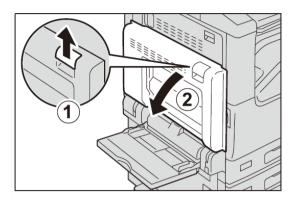
2. While lifting up the release lever, open the door C at the top part.
