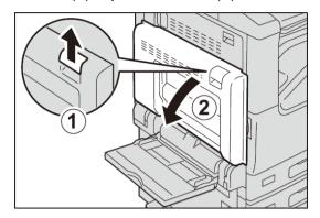
2. If paper is jammed outside the fusing unit, remove the jammed paper.
