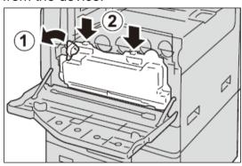
3. Put the new waste toner container into the device properly.
