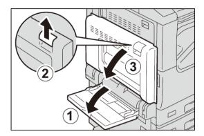
2. Lift up the lever A2, remove the jammed paper, and return the lever A2.
