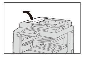
2. Turn the knob to transfer the jammed paper upward and remove it.
