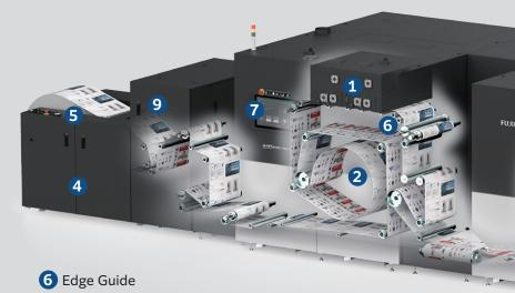
Paper movement, positioning monitoring allows for adjustment to remove any misalignment of the paper path which allows for a smooth printing process.
