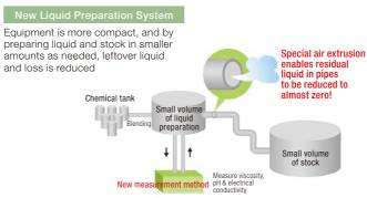
Measurement method which returns the liquid
