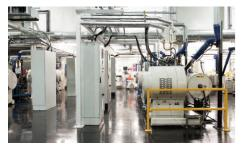
Ink mixing tank used in the clean, high-tech environment at the new factory
