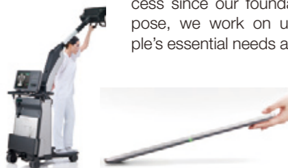
This compact mobile digital radiography system with excellent operability in a limited space was developed from direct observations made in emergency rooms. The panel to be inserted between the patient and the bed has a curved profile for easy insertion.
